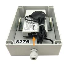
**6.** Check the status indicator on the BlipNode 5 minutes after power on.
