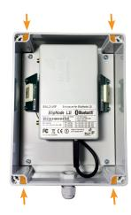
**3.** Ensure that the sensor is mounted according to the installation plan and the antennas (WF1 and WF2) are pointed in the right direction.
