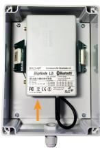
**5.** Check the status indicator on the BlipNode 5 minutes after power on.
